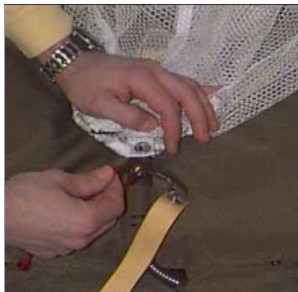
15. Pinning the pilot chute guide strap in place.
