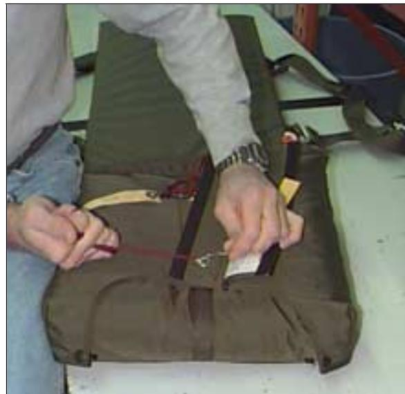
30. Pull the upper portion of the side flap into position while holding the top flap material in place.
