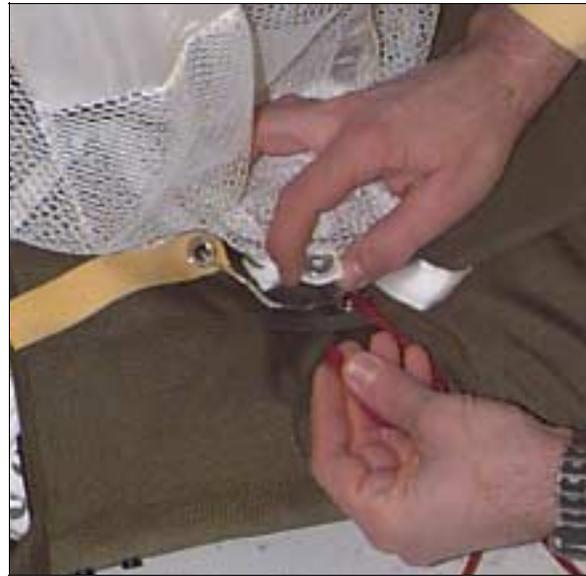
13. Holding the pilot chute in place, remove the temporary pin, pull the closing loop through the grommet on the guide strap, and pin in place.
