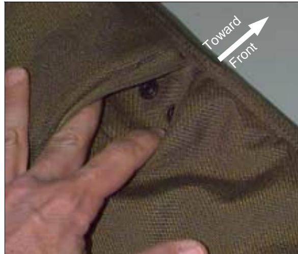
38. Containers that use the additional snap on cushion will have an extra snap on the front of the container. The outboard snap is used to hold the cushion in place. (Shown here prior to packing; you may unsnap the front corner snap if needed.)
