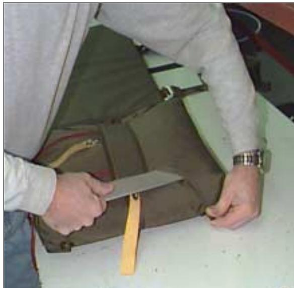
33. After removing any wrinkle, and keeping the corners as neat and full as possible, carefully close and snap the corners of the containers as shown. Use your finger to reach inside and poke the corner tuck out if needed.
