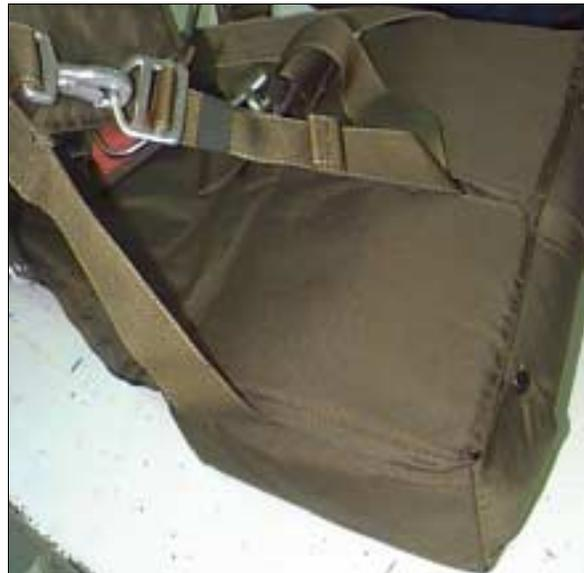
35. If the parachute you are working on is a BPS Warbird Seatpack model (extra 1" thick back pad), then the riser covers must be tacked above and below the horizontal back strap. These tacks prevent the riser covers from pulling open due to the extra back pad thickness. Using one turn single Super Tack or equivalent, tack through the binding tape of the riser covers and the back pad.
