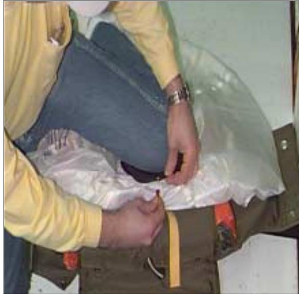
19. Being careful not to trap any material in the pilot chute spring, remove the temporary pin, pull the closing loop through the grommet in the pilot chute crown and re-insert the temporary pin.
