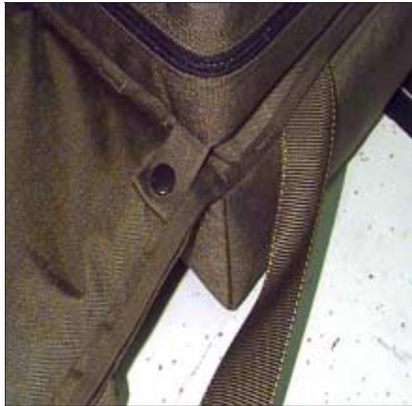
40. Unsnap the front corner container snap, snap the cushion to the outboard snap, and re-snap the container snap.
