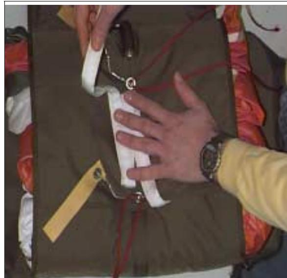
12. After "S" folding the pilot chute bridle, place the base of the pilot chute on top of the bridle. Holding the pilot chute in place, pass the bottom pull-up cord through the first grommet on the bottom pilot chute guide strap.
