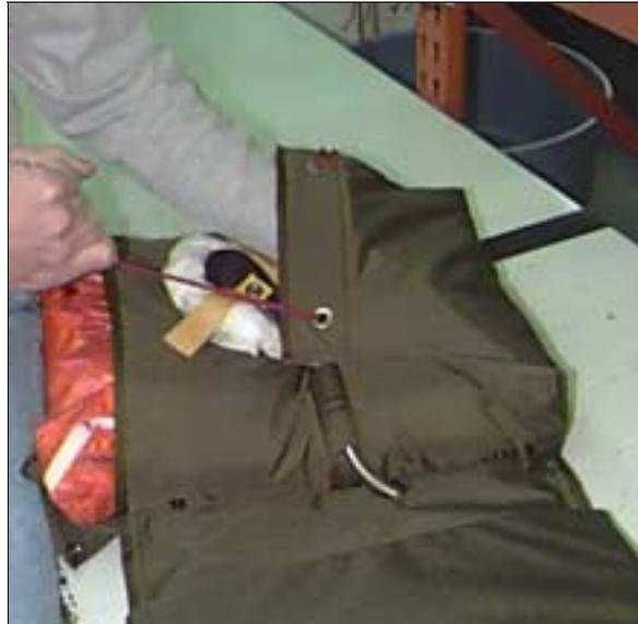
26. Once the side flap is in position, remove your temporary pin, pull the closing loop through the grommet, and pin in place.
