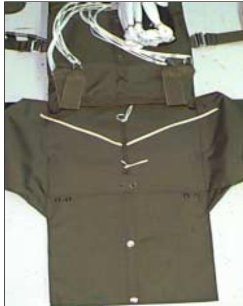
3. Place the canopy diaper across the front edge of the pack tray and position the risers as shown. Using the approximately 20" of suspension lines that were left unstowed, form a bight in the lines and secure to the pack tray with the 12" piece of 80 Lb cotton break tape using a Surgeon's and locking knot. Trim the 80 Lb 1" from the ends.
