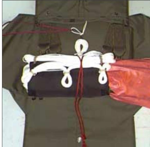
5. Bring the bottom container flap up and over the diaper, route the bottom pull-up cord through the appropriate grommet, and pin in place with a temporary pin.
