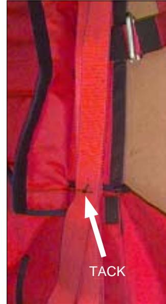
2. After tacking the risers into position and closing the riser covers, insert a 12" piece of 80 Lb cotton break tape under the Type IV webbing located in the center of the pack tray. This will be used to secure the first bight of suspension lines to ensure proper staging of the canopy during deployment. Next, insert your pull-up cords into the container closing loops.
