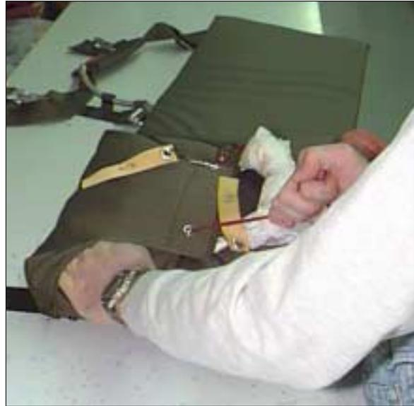
28. Close the right side flap in the same manner as the left. Hold the top flap material in place while pulling the side flap into position...
