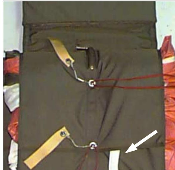
11. With the top and bottom flaps closed, begin stowing the pilot chute by "S" folding the pilot chute bridle between the grommets on the top flap. As you fold, spread the bridle out to eliminate bulk, but keep it in the area under the center of the pilot chute spring.
