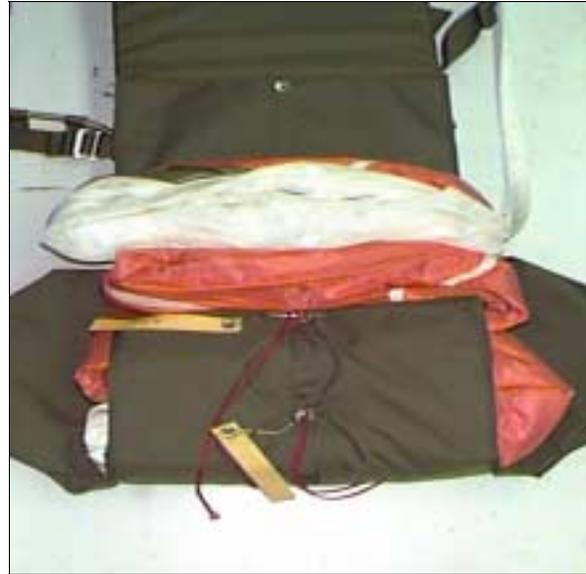
10. Fold the top flap over the bottom flap, route your pull-up cords through the grommets, and pin in place. Ensure that the pilot chute bridle is properly routed out from under the top flap (arrow).
