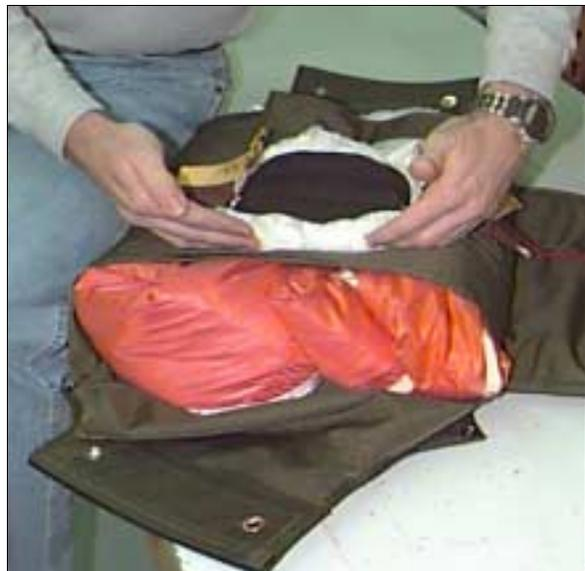
24. Begin closing the container by routing your pull-up cords through the grommets on the left side flap.
