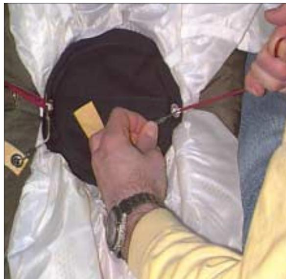
21. With the pilot chute securely in place, carefully fold the remaining pilot chute
