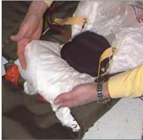
22. ...And tuck it around the sides of the pilot chute crown. Position this bulk so that it prevents the pilot chute spring from wobbling or rocking. You must also ensure that the pilot chute cloth is not trapped under the side flaps when the container is closed.
