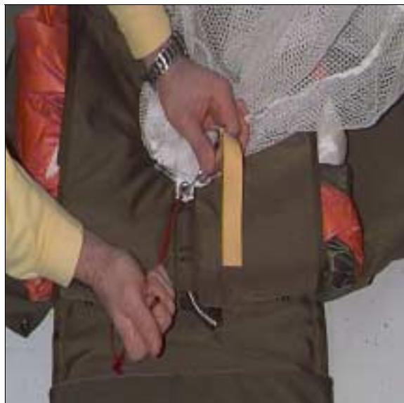
16. Carefully compress the pilot chute and pull all the material (mesh and cloth) clear of the spring.
