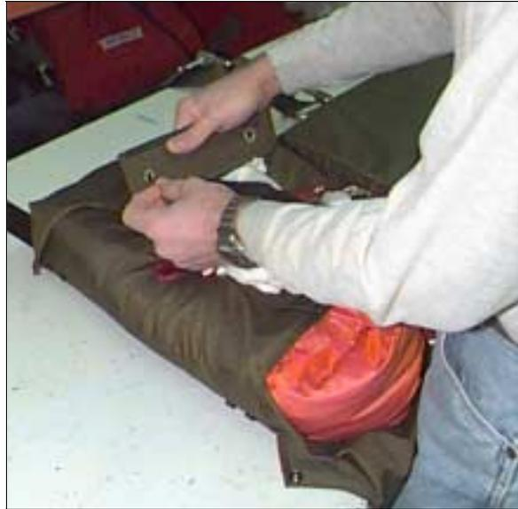
25. Using one hand to hold the top flap material in place (to prevent wrinkles) begin pulling the side flap into position.
