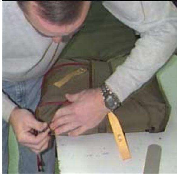
34. Ensure that there are no twists in the leg straps, then snap the "V" rings in place. If the leg straps were not in place for some reason, carefully slide them through the slots as shown here, then snap in place.
