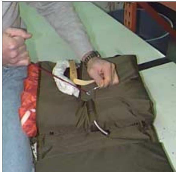
27. Again using one hand to hold the bottom flap material in place, pull the side flap into position and pin in place. Take care to push any wrinkles (in the top & bottom flap) to the outside.
