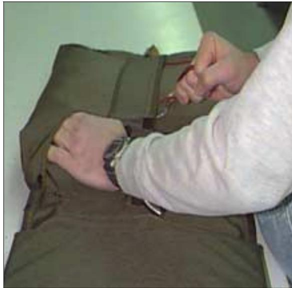
31. Complete closing the container by pinning the side flap in place.
