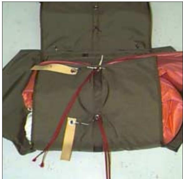
9. "S" fold the remainder of the canopy into the pack tray. Folding the apex back towards the center will place the pilot chute bridle in the correct position and leave a cleaner edge when closing the container. Again, pay attention to the amount of canopy that is placed under the ripcord housing.
